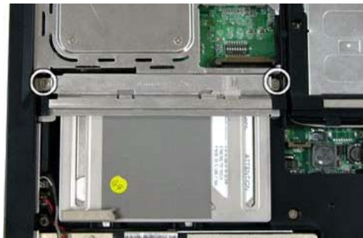
Fig. 14 Removing the hard disk drive screws
